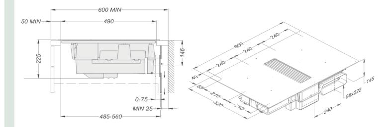
\*When installing directly against an uninsulated outside wall, we recommend using an installation kit with air outlet in the plinth.
